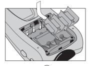
3 Insert the battery pack (included with the recharging dock) as indicated on the side of the battery pack.
